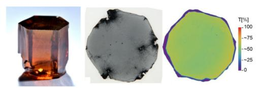
Figure 1: AlN bulk crystal, Ø 10 mm (left). X-ray transmission topograph (middle) and map of optical transmission at 254 nm (right) of a 140  $\mu$ m thick AlN substrate with Ø 10 mm.
